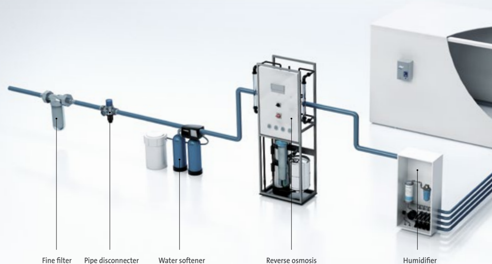
Schematic diagram of a water treatment system for adiabatic humidification
