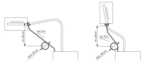
Lead the condensate hose down to the humidifier with a **minimum slope of 20** %, in the form of a **siphon (min. hose bend diameter \emptyset200 mm )**. Then, lead the hose into the unit through the break-through on the top side of the unit and insert it about 2 cm into the specified opening of the water cup.
