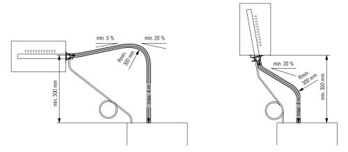
Initially, lead the steam hose with an **upslope of at least 20% over a minimum height of 300 mm** above the top edge of the unit, then lead the hose with a **minimum upslope of 20%** and/or a **minimum downslope of 5%** to the steam distribution pipe.
