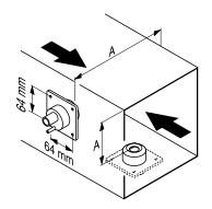
The **steam nozzle W21** can be mounted in the ventilation duct horizontally or vertically. Keep a **minimum distance clearance (A) of 200 mm** between nozzle opening and the opposite duct wall.
