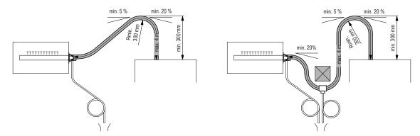
Initially, lead the steam hose with an **upslope of at least 20% over a minimum height of 300 mm** above the top edge of the unit, then lead the hose down to the steam distribution pipe with a **minimum slope of 5 %**.
