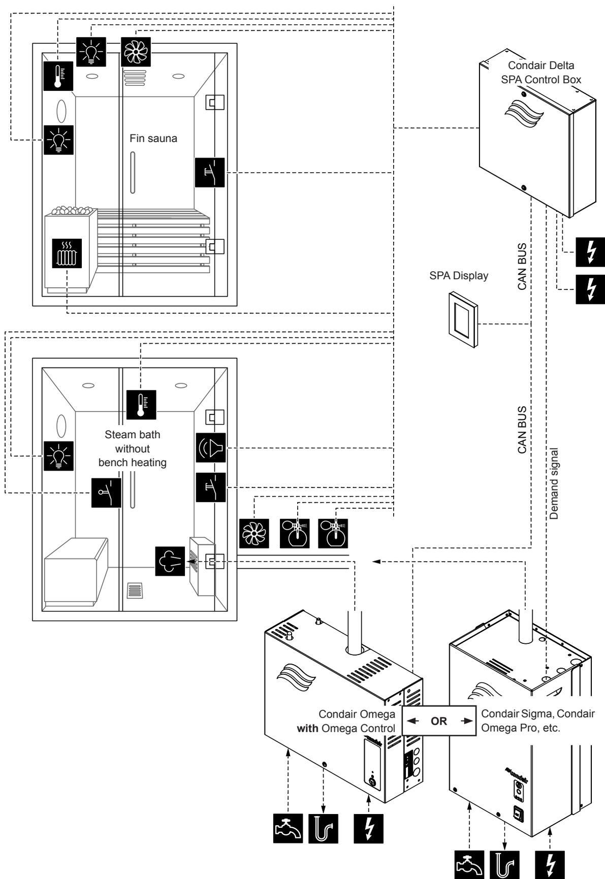
Fig. 11: Condair Delta SPA Control Box for dual cabin applications for small cabins
