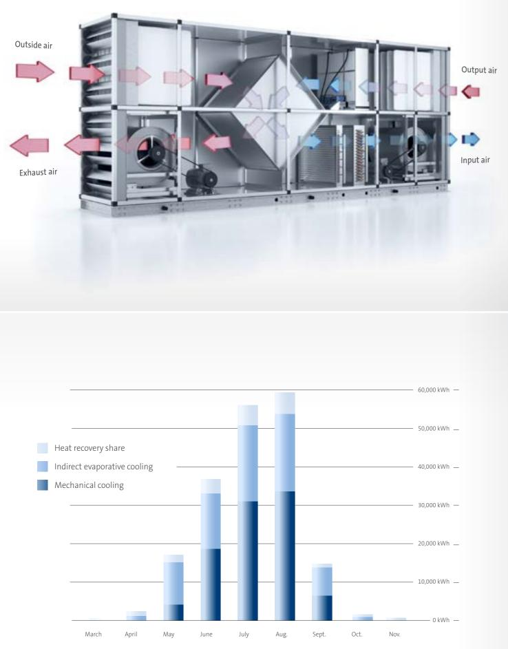
Graphical representation of energy contributions produced for the cooling of buildings in the sample air conditioning system. Calculated using the Coolblue 2.0 software tool from Condair.
